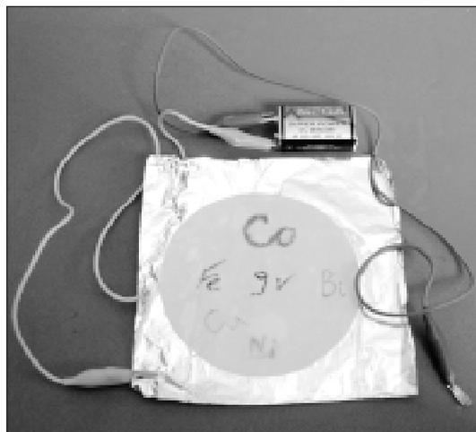
Figure 6. Marks on filter paper soaked with potassium thiocyanate, written with Fe, Cu, Ni, Co and Bi anode
