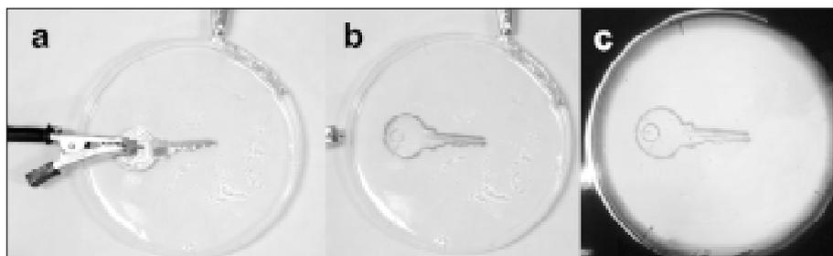
Figure 4. Experiment with phenolphthalein gel: key anode (a), mark obtained after some time (b), projection (c)
