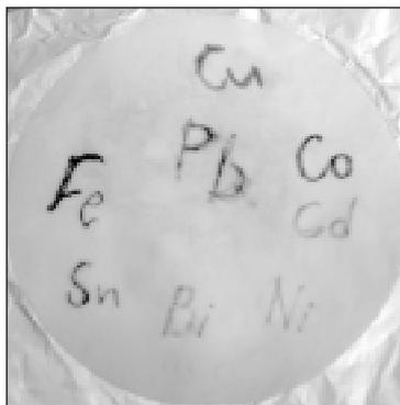
Figure 7. Marks on filter paper soaked with sodium sulfide, written with Cd, Sn, Fe, Pb, Cu, Ni, Co and Bi anode
